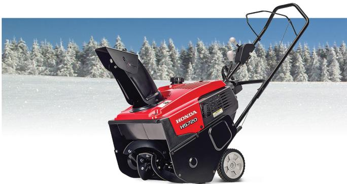
**Single-stage** are lightweight, compact and ideal for light to moderate snow conditions (less than 20 cm [8 in.]). They are designed to handle small jobs like sidewalks, walkways and short driveways. Single-stage snowblowers rapidly take in snow and direct it through a discharge chute in a single motion, hence the name, single-stage. The auger (the blade you see in front of the blower) makes contact with the surface you are clearing and therefore should only be used on paved surfaces.
