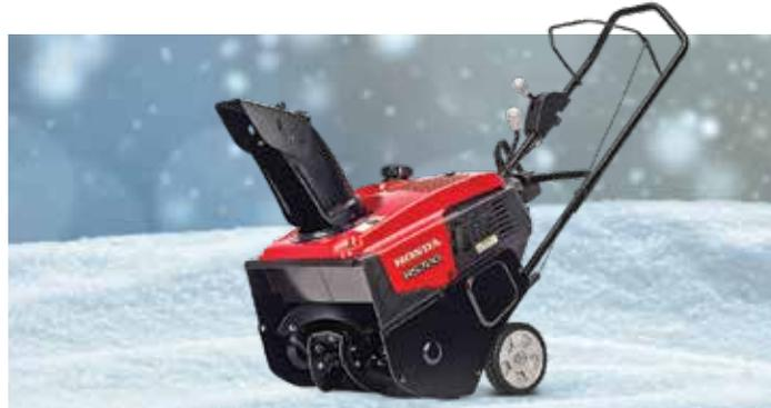
**Single-stage** are lightweight, compact and ideal for light to moderate snow conditions (less than 20 cm [8 in]). They can handle small jobs like sidewalks, walkways and short driveways. Single-stage snowblowers rapidly take in snow and direct it through a discharge chute in a single motion, hence the name, single-stage. The auger (the blade you see in front of the blower) makes contact with the surface you are clearing and therefore should only be used on paved surfaces.
